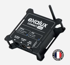
**EXALUX™** CONNECT ONE already has its own Wi-Fi and Art-Net/DMX interface so it works without the need of an extra access point. CONNECT ONE can be directly powered from AC line or with an external battery. It can run up to 12 hours with the small 8.5Wh Exalux Powerbank. Swaping from one power supply to another does not disconnect Wi-Fi connection.
